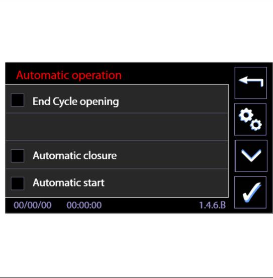
**If the CB7015 automatic system is installed, the recommended setup for the Automatic Operation function is with all options enabled, as shown here.**
